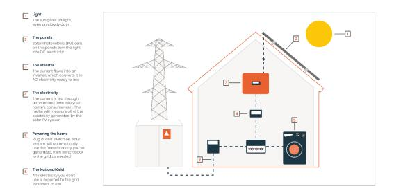
Solar PV systems use cells to convert sunlight into electricity. The PV cell consists of one or two layers of a semi conductive material, usually silicon. When light shines on the cell it creates an electric field across the layers causing electricity to flow. The greater the intensity of the light, the greater the flow of electricity.
